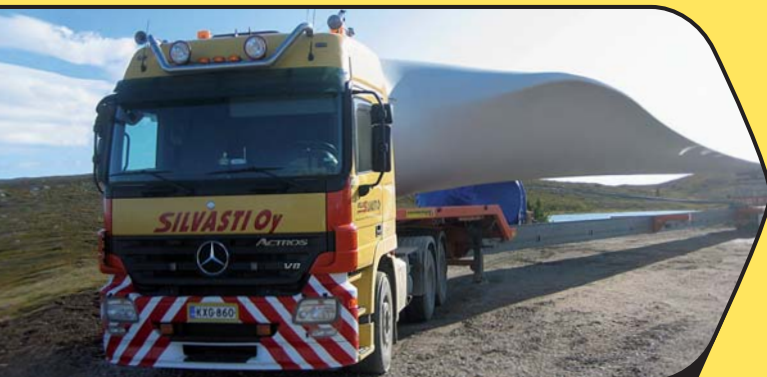
One of the Silvasti's triple extendable blade trailers. Silvasti's equipment can transport blades up to 60 meters.
