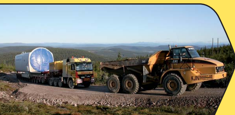
Total weight of this truck carrying nacelle is over 200 tons, so dumber truck was needed to assist the truck on top of the mountain.
