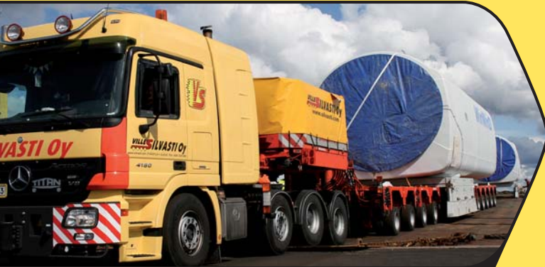
All four nacelles were transported at the same time by barge from Loviisa, FIN to Skellefteåhamn, SE and by Silvasti's heavy equipment to the site.
